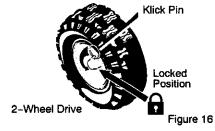
For ease of maneuverability in light snow conditions, disconnect the klick pin from the wheel locked position and push into the single wheel drive position (unlocked axle hole only). See Figure 17.
